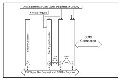
Figure 1-3. PXI Star Trigger and Local Bus Routing
